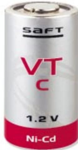
The VT C cell is designed to accept a permanent charge (C/20) for a minimum of 4 years in high temperature environments (up to + 55°C) such as security lighting installations.
