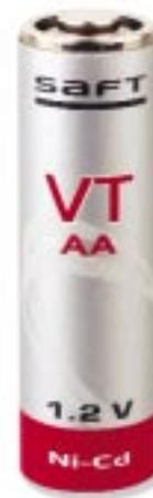
The VT AAH cell is designed to accept a permanent charge (C/20) for a minimum of 4 years in high temperature environments (up to + 40°C) such as security lighting installations.
